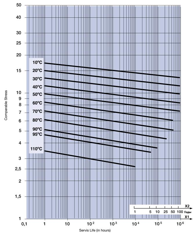
The regression curve shows an impressive long term resistance at high temperatures and indicates the service life cycle.
